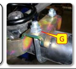
Step 3: Install MetalCloak Track Bar (or Reinstall Stock Track Bar)
