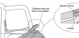
Manufacturing Note: Due to a recent header assembly modification by Daimler Chrysler, the plastic strip on the windshield header may have 8 screw locations instead of 14. Both attachment numbers of screws will securely fasten the header and perform as the original design was intended.
