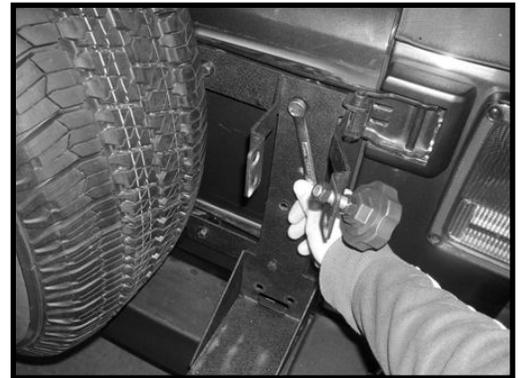
4. If installing Off Road Mounting Bracket with a RR tire carrier, secure the mounting bracket to the lower mounting plate's top two holes using M10 hardware as shown. The upper mounting plate can now be rotated into its horizontal position to line up with the mounting bracket's middle hole and the upper right tailgate hinge hole. Insert the remaining M8 hardware and tighten. Go back and make sure all bolts are tightened before inserting your Off Road Jack.
