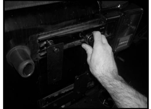
If no RR tire carrier is present, rotate the bracket installed in step 2 into its vertical position and the upper mounting plate into its horizontal position. Line up the holes in the plate and the bracket with the upper right tailgate hinge hole. Tighten the bracket into place using the remaining M8 hardware as shown. Also, fully tighten the bottom right tailgate hinge bolt.
