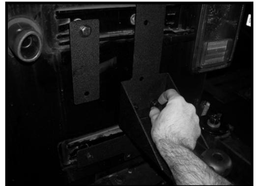
If installing Off Road Mounting Bracket without a RR tire carrier, install the final M10 bolts into the bottom holes in the mounting bracket as shown. Go back and make sure all bolts are tightened before inserting your Off Road Jack.
