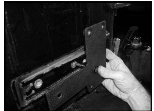
If installing on a vehicle without a RR tire carrier, the mounting bracket should be installed with the lower mounting plate in this step. Line up the bottom M8 hole with the bottom right tailgate hinge bolt hole and insert M8 hardware as shown. Do not fully tighten the bolt securing the mounting bracket. The mounting bracket will have to be rotated to gain access to the upper right tailgate hinge bolt in the next step.
