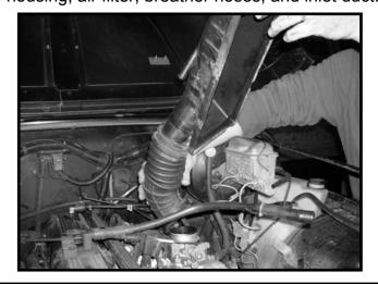
2. Remove rubber grommets from the air filter housing. Mount and install Heat Shield in place using 1/4-20 hardware.
