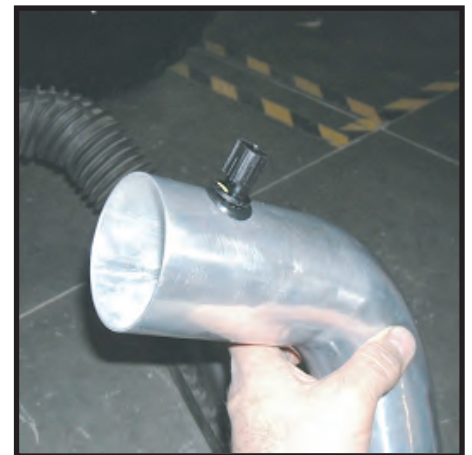
Install sensor into new tube
