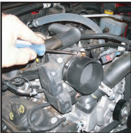
Install throttle body coupling
