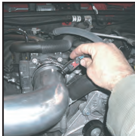
Lead connected to temp sensor
