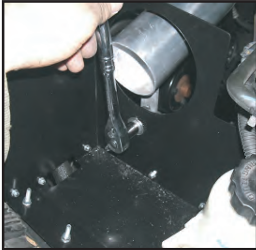
Secure tube to heat shield
