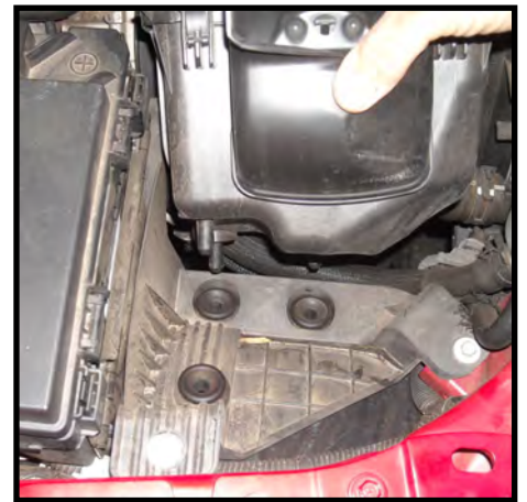
Pull air box free from inner fender
