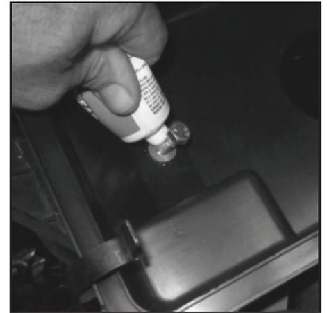
**61** - Install (2) M8 Nuts and (2) M8 flat Washers to the underside of inner fender mounting plate. Add sealant if needed to insure a water tight seal.
