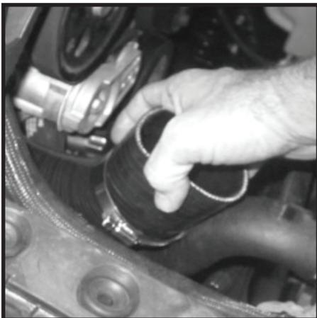
**50** - Trim just enough of the 90deg Elbow for the Air Box to rest within 1/8" (3mm) of rubber grommets. Repeat step (48) making small adjustments to 90deg Elbow until fit is correct.
