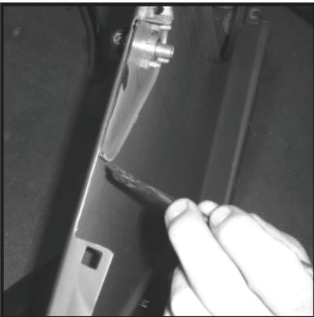
**38** - Apply a very small amount of super glue to inner corners of "U" Gasket. It will be easier to start at on end and work around opening applying glue as needed. This will insure "U" Gasket remains in place during reassembly.
