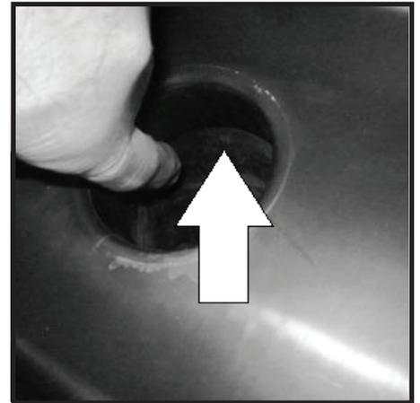
**55** - Apply a thin film of sealant around end of Air Tube. An excessive amount may cause the elbow to slide off air tube when tightened.
