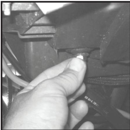
**62** - Tighten M8 hardware to secure new Air Box to vehicle. Inspect sealant around bolt heads and washers to insure there are no gaps. Smooth out sealant and clean off extra material.
