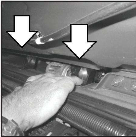
**77** - Locate Cowl Nut Plate. Nut plate is used to secure cowl cover and snorkel body to Cowl "Z" - Bracket.
