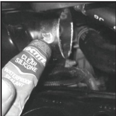
**56** - Apply sealant to the inside of two lower rubber grommets as shown. Make sure sealant completely fills the two holes.
