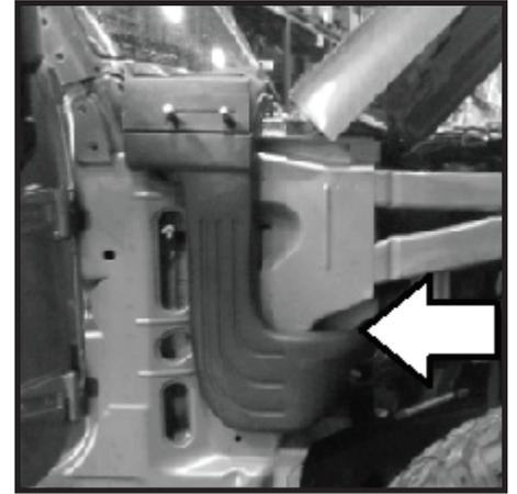
**73** - Inspect Cowl "Z"-Bracket to Main Body alignment. Adjust Main Body and Cowl "Z"-Bracket to align mounting holes. If needed Cowl "Z"-Bracket can be adjusted (bent) to align all holes.
