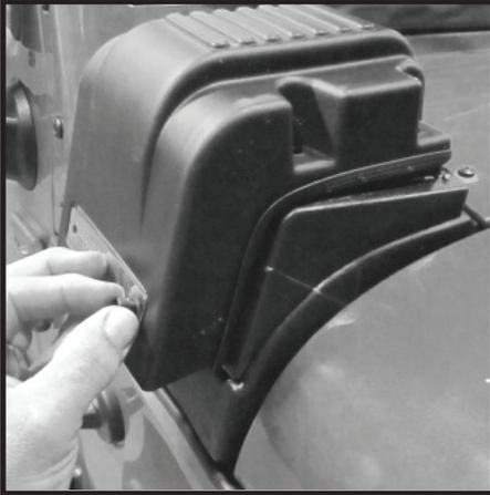
**89** - Press top of Low Mount Air Intake down onto Main Body. Intake will fit over top front of main body intake and pop over the rear of intake as shown.
