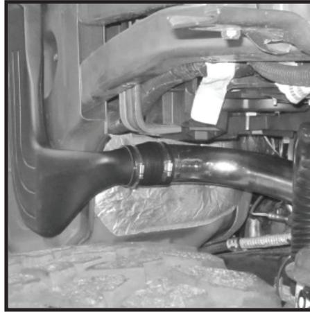
**72** - Snorkel Main Body should rest in place as shown. Snorkel Main Body should be fitted tight to inner frame. Some vehicles may require the pinch seam (arrow) to be rolled for proper fit. Check antenna cable position.
