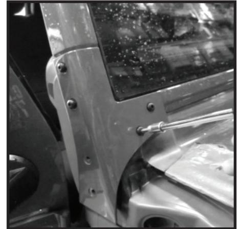
**67** - If used, windshield light mounting brackets should be installed at this time. NOTE: the snorkel system has been designed to work with most Rugged Ridge components. Rugged Ridge cannot guarantee that other manufactures components will work or clear the XHD snorkel system.
