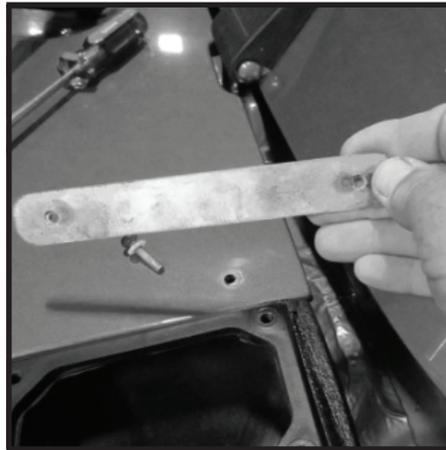
**78** - Slide Cowl Nut Plate under Main Body as shown. Working from engine compartment align mounting holes. Start one M6 Phillips head screw to hold in place.
