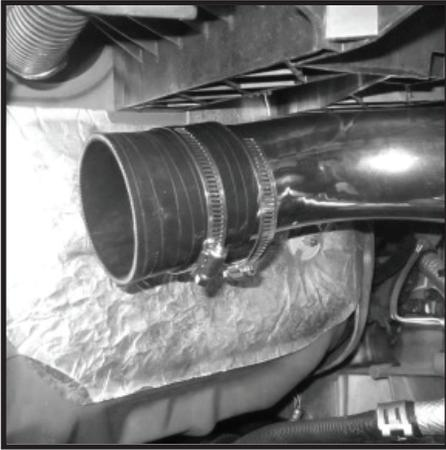
**71** - With sealant applied to main body outlet slip Hose Clamp onto Main Body outlet. Position snorkel Main Body onto vehicle sliding outlet into Coupling as shown. Slide Hose Clamp over Coupling but Do Not tighten.
