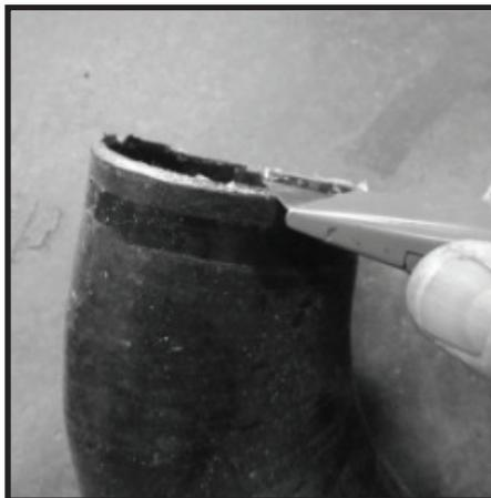
**51** - With Air Box in the correct location, 90deg Elbow attached to lower Air Box inlet and aligned with the Air Tube. Carefully remove Air Box and 90deg Elbow together. Mark the position of the 90deg Elbow to Air Box as shown. remove elbow for step (52).
