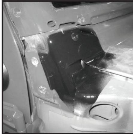
**66** - Install windshield bracket removed in step (2). Start and tighten upper side M12 bolts and front M12 bolts as shown. Windshield brackets can be adjusted. If needed a screw driver can be used to loosen windshields floating nut plates. This will allow for realignment of plate.
