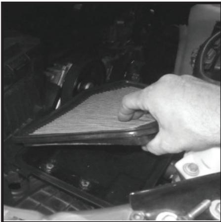
**86** - Reinstall factory upper air box removed in step (42). Rotate 3" intake hose back onto upper air box and secure factory hose clamp.
