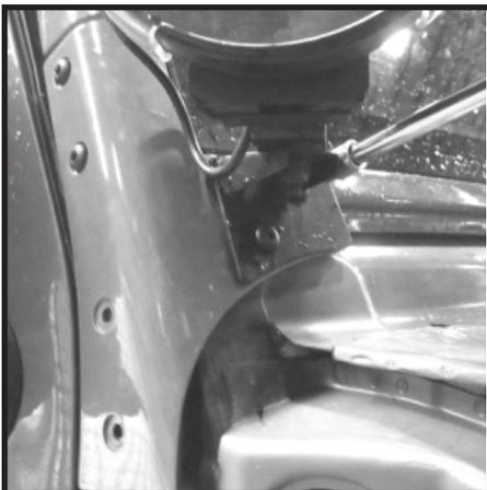
**68** - Install Cowl "Z" Bracket plate reusing factory 10mm bolts removed in step (9). Secure the bolts but do not tighten at this time. Adjustment to main body will be required during install.
