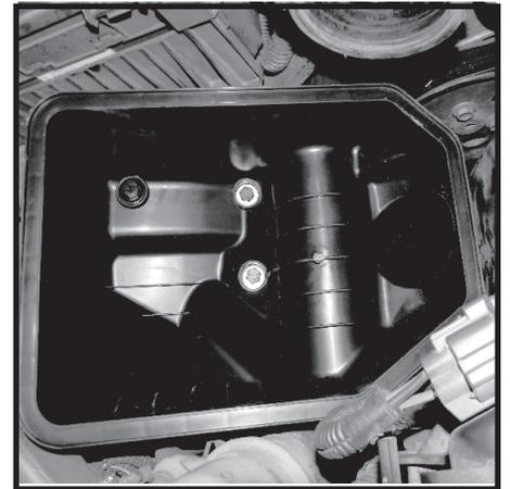
**49**- If Air Box does not fit within 1/8" (3mm) of rubber grommets the top of the silicone 90deg Elbow will need to be trimmed. Remove Air Box and 90deg Elbow. If Air Box fits correctly proceed to step (51).
