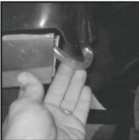
**92** - Add "U" Gasket to low mount intake if not already installed to snorkel main body. Starting from lower intake edge work around the intake making sure gasket is fitted tight to intake. Trim gasket if needed.
