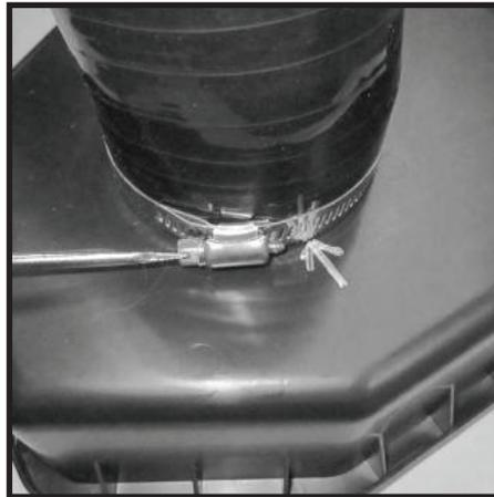
**54** - add extra sealant to the inside lip of lower Air Box inlet and 90deg Elbow as shown. Extra sealant can also be added to the outside as well.
