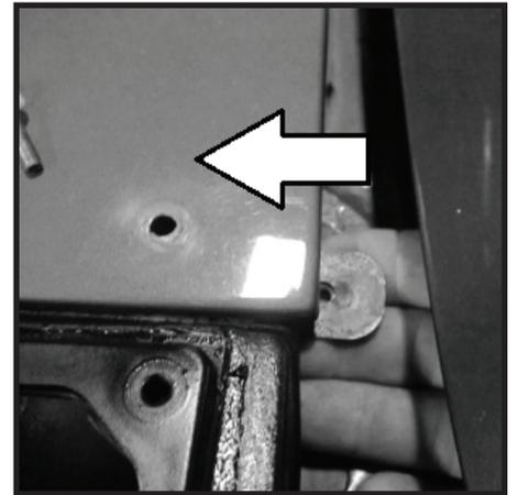
**79** - Secure all (4) M6 cowl mounting screws. Make sure M6 black washers are placed under M6 screws before tightening.
