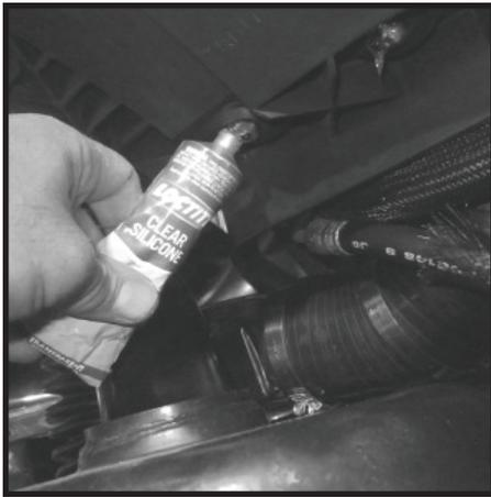
**59** - Reinstall lower Air Box and 90deg Elbow. Slide 90deg Elbow over Air Tube. Apply extra sealant around outer edge of the 90deg Elbow and Air Tube. Slide Hose Clamp over 90deg Elbow but do not tighten at this time.
