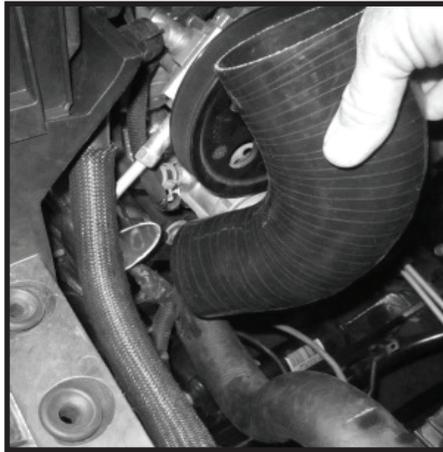
**48** - Place new Air Box onto 90deg Elbow. Making sure elbow is fully seated to Air Box inlet. Air Box should rest within 1/8" (3mm) of rubber grommet.
