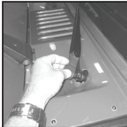
**81** - With Main Body installed inspect Air Tube. Tighten 10mm bolt at Air Tube mount and brake bracket.
