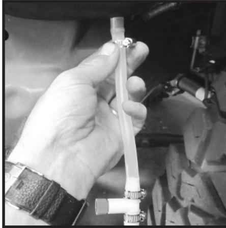
**84** - Drain Hose should be cut into two lengths. Top section should be about 8" long. The lower section will be 4" and trimmed as needed. Connect 3/8" Hose Clamps to 3/8" Drain Valve and tighten all clamps.
