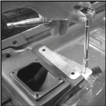
**74** - Place windshield cowl cover back onto vehicle. Align driver's side top holes and insert (2) M6 x20 Phillips head screws and washers. Secure but do not tighten.
