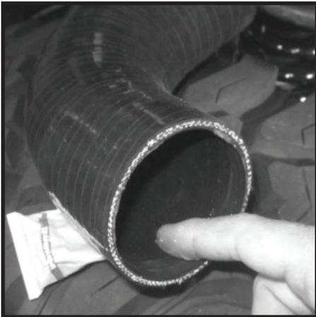
**53** - Reinstall 90deg Elbow to Air Box. Align marks made in step (51). Slide hose clamp onto elbow. With 90deg Elbow placed against bottom face of Air Box tighten Hose Clamp. Pull on 90deg Elbow to insure it is secured tightly to inlet.
