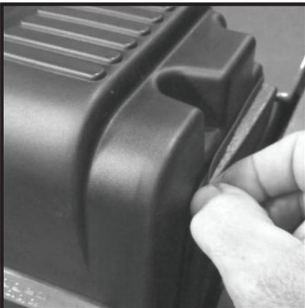
**92** - Tighten all (6) caps head bolts. Do Not Over Tighten. A firm seal is all that is required.
