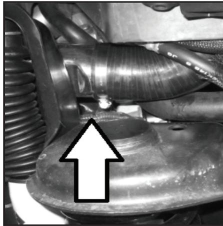
**60** - Insert (2) M8 x 35mm Bolts with (2) M8 Flat Washers through Air Box mounting holes and rubber grommets. Apply a small amount of sealant to washers.
