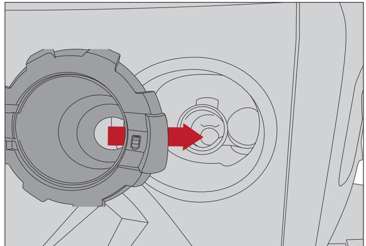
6. Reattach fuel door tether to Rugged Ridge Fuel Door filler housing.
