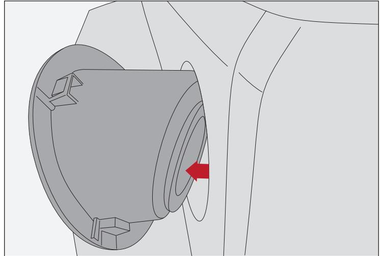
5. Align grommet on filler housing with fuel filler. Apply moderate pressure to front face of fuel door to engage.
