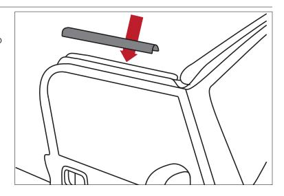
5. Unfold Soft Top and set windows aside, taking care not to scratch windows. Place top on center of roll bar and unfold. Spread top out, taking care that metal flat hooks at end of rear adjustment strap do not damage paint, glass, or cause injury.
