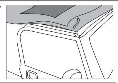
6. Insert front plastic into groove of Windshield Channel. Ends will match nearly to each end of Windshield Channel. From front of vehicle, ensure that top is even from side to side. Check door surround sides and push top toward rear to ensure fabric is seated tightly around front corners.
