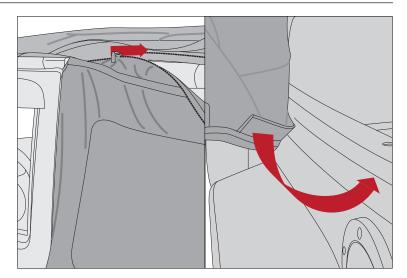
11. Before continuing, ensure rear door zippers have been started on both sides. Set Belt Rail plastic even with factory weather strip at body gutter directly behind door. Continue fastening plastic under Belt Rail lip of body until top is fully attached around back corners of body.
