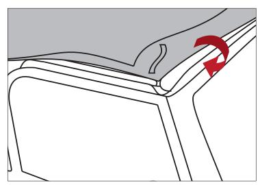
7. Insert plastic into top of door surround channels above either door opening. This will center top at front. Check that front plastic is near front of windshield channel.
