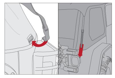
15. Bows are easily installed and removed by pushing forward and into or back and out of pocket.
