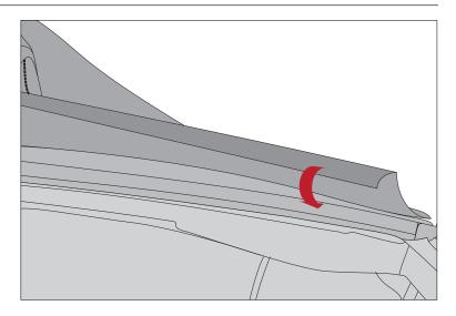
8. Locate ceiling adjustment straps at rear corners on ceiling panel. Gently pull strap over rollbar and around seatbelt stud and back up to strap adjustment buckle. Tighten snugly and repeat other side. Check top for evenness from side to side.
