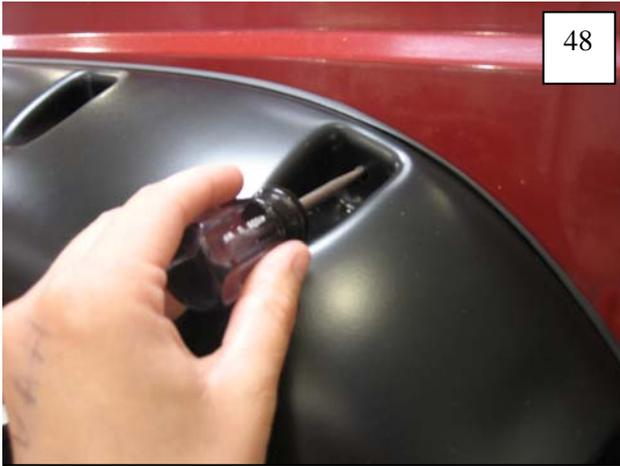
Hold the Rear Main Flare on the fender, aligning with door seam and fender contours. Press firmly. Using the holes in the part as a guide, mark hole locations on fender (5 places).
