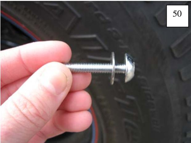
Place a supplied washer onto a supplied Torx head screw.
