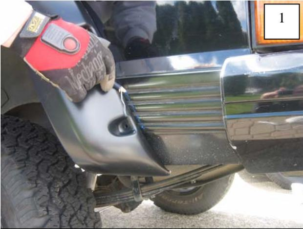
Prior to marking hole locations, hold the Flare on the fender, pressing firmly. Making sure the flare is properly positioned, trace the outline of the flare on the factory trim.
