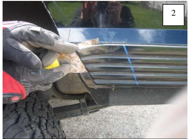
Use a putty knife to separate the factory trim from the fender, stopping at line made in Step 2.
