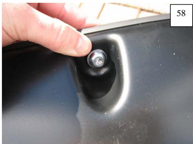
Insert screw and washer through each pocket in flare.
