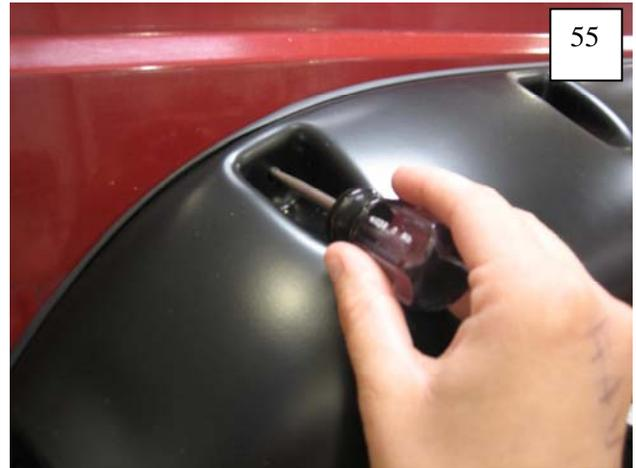
Using the holes in the part as a guide, mark hole locations on fender (4 places).
