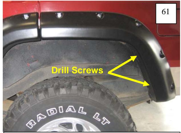
Optional: There are extra drill screws supplied in the kit. If desired, further secure the rear of the rear flare using drill screws. Place drill screw on part and drill into sheet metal.
