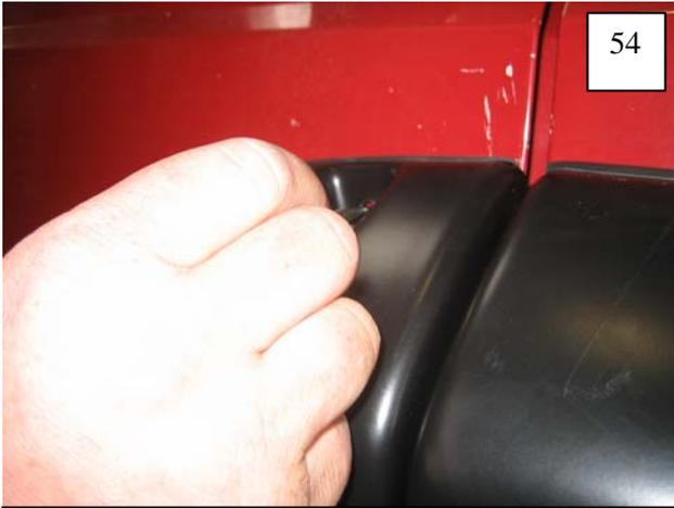
Hold the Rear Door Piece on the door, aligning with the Rear Main Flare. Press firmly to ensure proper hole location alignment.
