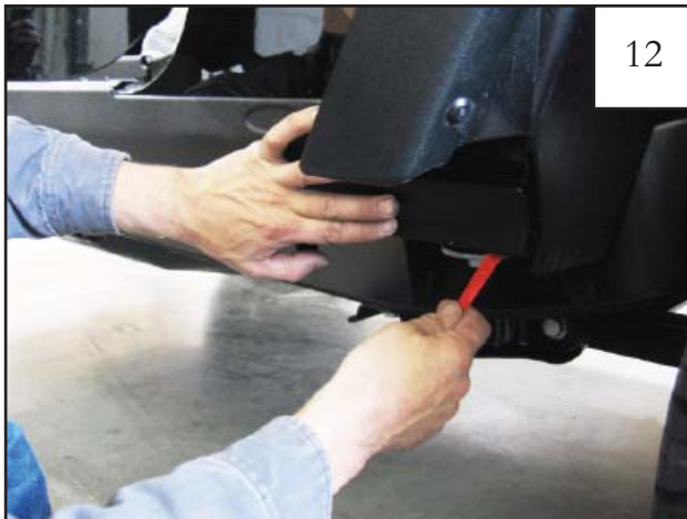
From rear to front, pull tape liner tab 7. Press firmly on the part following tape liner removal. NOTE: Refer to step 1 for additional tape tab identification.
