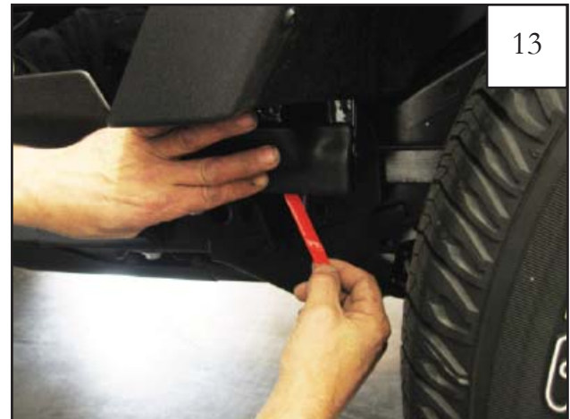
From rear to front, pull tape liner tab 8. Press firmly on the part following tape liner removal. NOTE: Refer to step 1 for additional tape tab identification.
