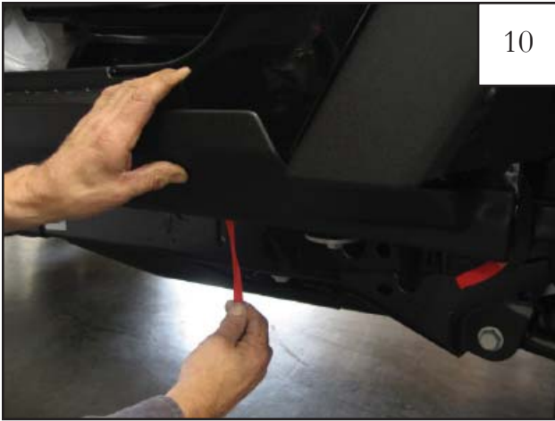
From rear to front, pull tape liner tab 5. Press firmly on the part following tape liner removal. NOTE: Refer to step 1 for additional tape tab identification.
