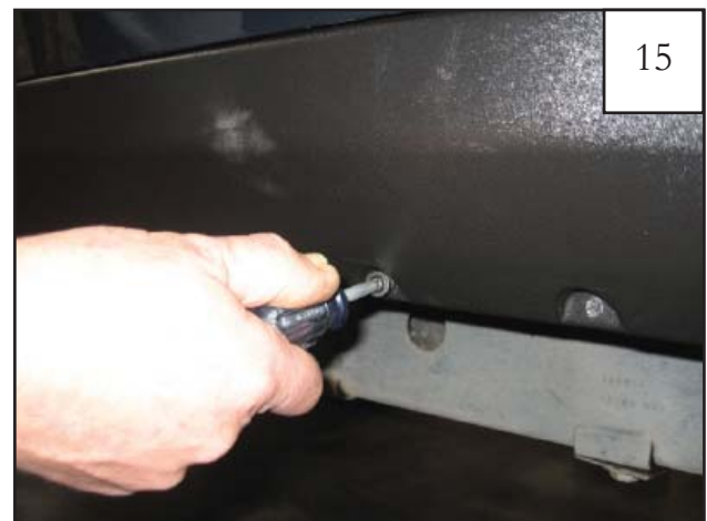
Using a #2 Phillips screwdriver, start a screw through each hole in side panel and through clips installed in step 4. Once all screws are started, tighten.
