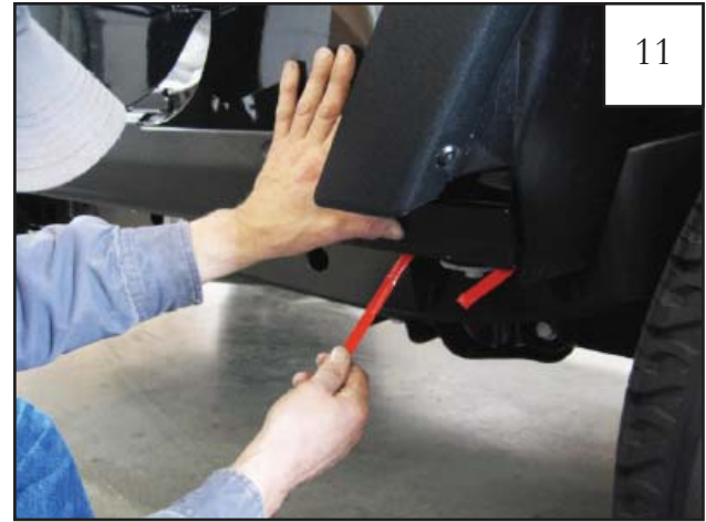
From rear to front, pull tape liner tab 6. Press firmly on the part following tape liner removal. NOTE: Refer to step 1 for additional tape tab identification.
